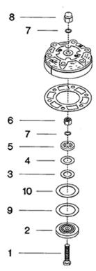
FIGURE 3. HIGH PRESSURE CONCENTRIC RING VALVE.
